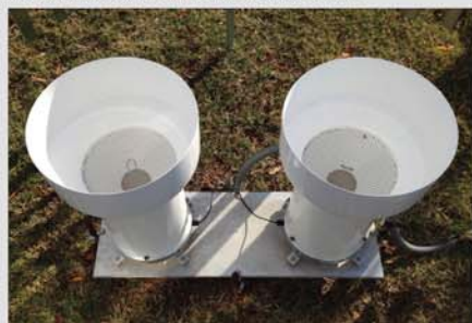
Dual rain gauges from Oklahoma Mesonet site
