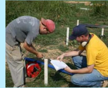
Garey Fox (right) and John Fuchs (left) measuring water level depth in the piezometers
