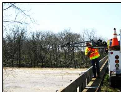
USGS Hydrologic Technician measuring streamflow during a flood on the Illinois River.
