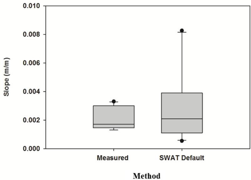
Figure 1.12. Channel bed slope calculated from the topographic map and aerial images (measured) and digital elevation model (SWAT default) for the Barren Fork Creek.
