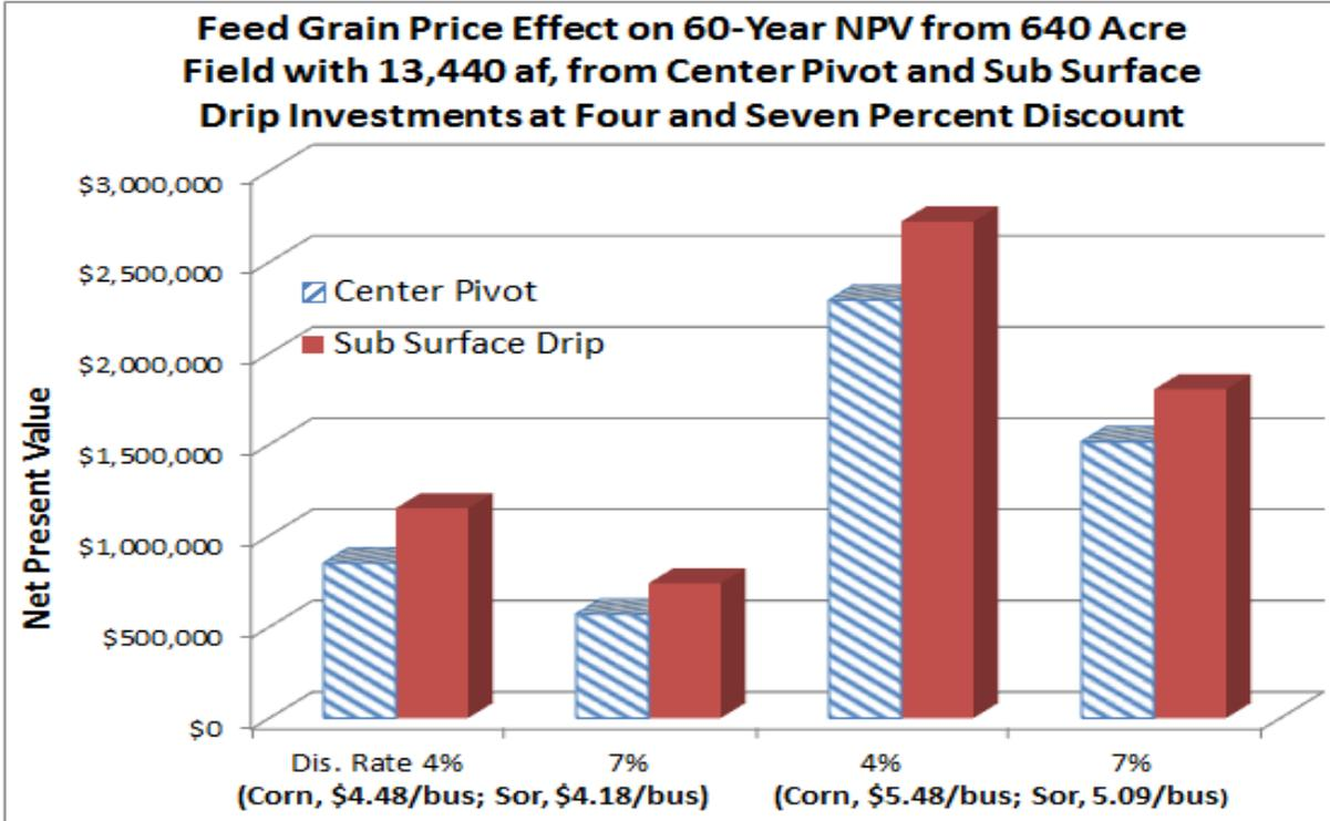
**Figure 30. Comparison of NPV from Center Pivot and Subsurface Drip Investments on a 640 Acre Field with Initial Water Supplies of 6,240 and 13,440 Acre Feet Under Two Feed Grain Prices and Two Discount Rates.**
