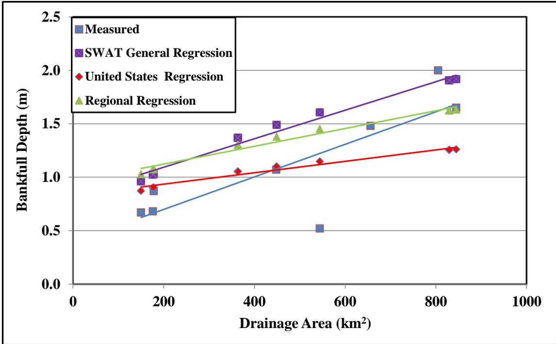
Figure 1.15. Measured bankfull depth and calculated bankfull depth using three empirical equations vs drainage area for the Barren Fork Creek.
