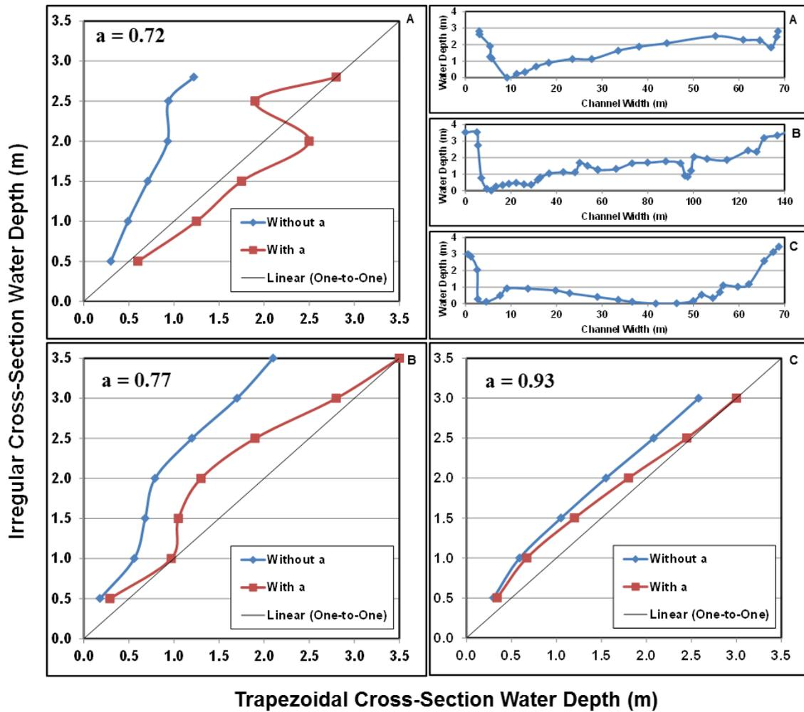
Figure 1.10. FlowMaster-calculated flow depth for the irregular cross-section compared to the trapezoidal cross-section with and without the area adjustment factor ( $a$ ). Cross-section A is a meander, B is a heterogeneous straight reach and C is a homogenous straight reach.
