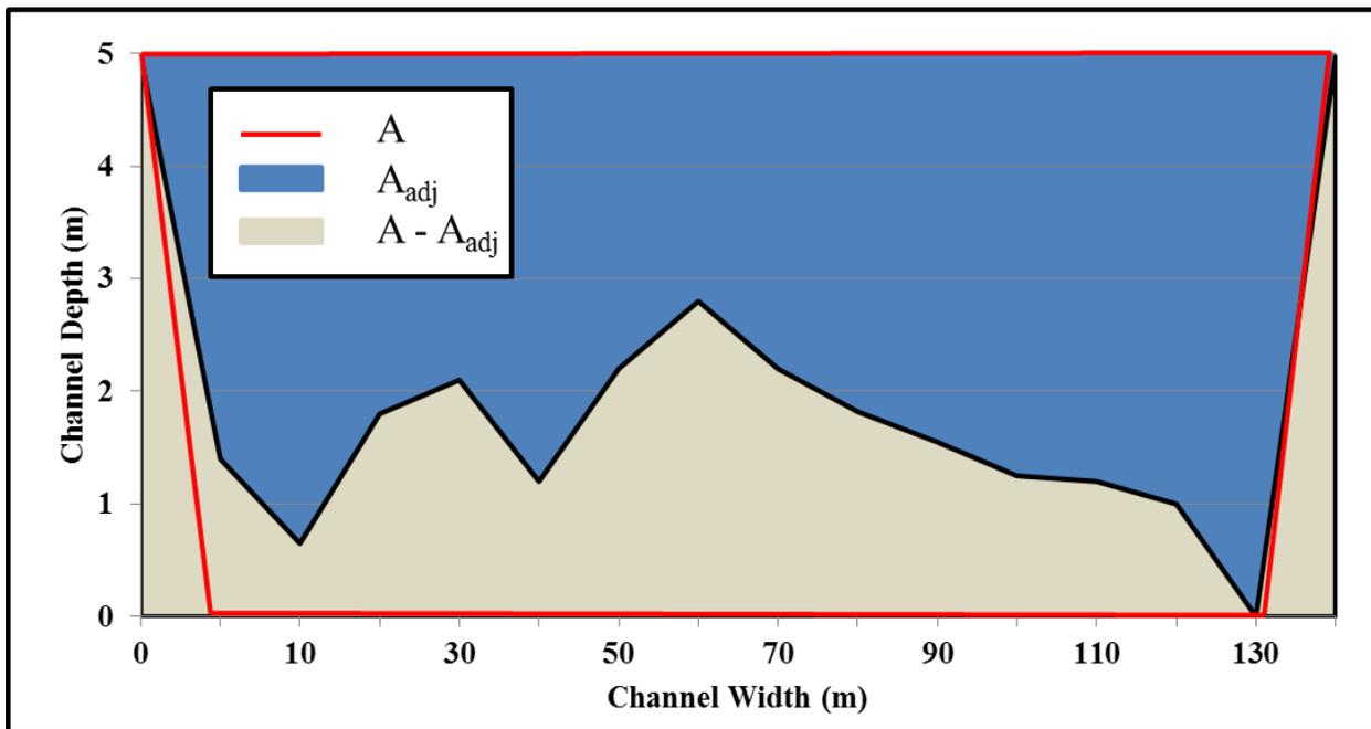
Figure 1.2. SWAT trapezoidal and measured stream cross sections at the United States Geological Survey gage station 07197000 used to adjust cross sectional area and calibrate flow depth.  $A_{adj}$  is the measured cross-sectional area of the natural channel,  $A$  is the cross-sectional area of an assumed trapezoidal channel,  $A - A_{adj}$  is the difference between the trapezoidal and measured cross sections.
