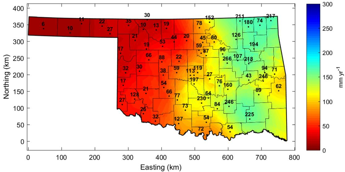
**Figure 1. Statewide mean annual soil moisture-based drainage rates for the years 1998-2014 in mm per year. Drainage rate labels for the Stillwater, Oklahoma City East, Porter, and Marena sites were excluded for clarity, but were 214, 82, 166, and 66 mm yr<sup>-1</sup>, respectively.**
