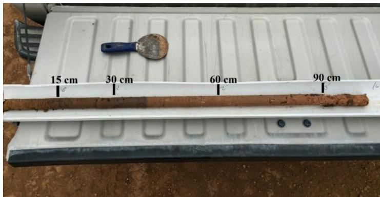
Figure 3. soil core and sub-cores lengths
