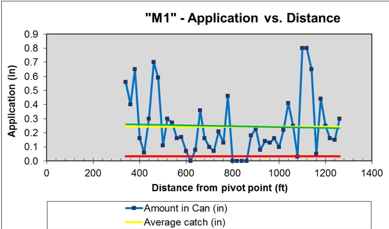
**Figure 8:** Water application amount at distances from pivot
