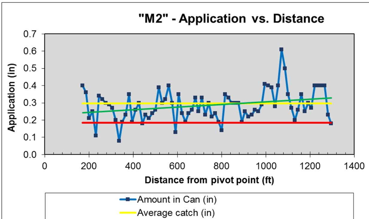
Figure 9: Water application amount at distances from pivot
