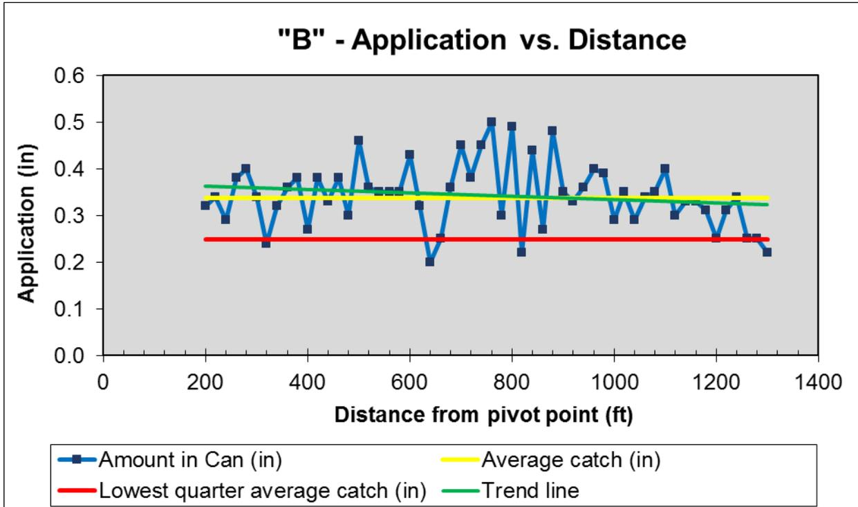
**Figure 6: Water application amount at distances from pivot**
