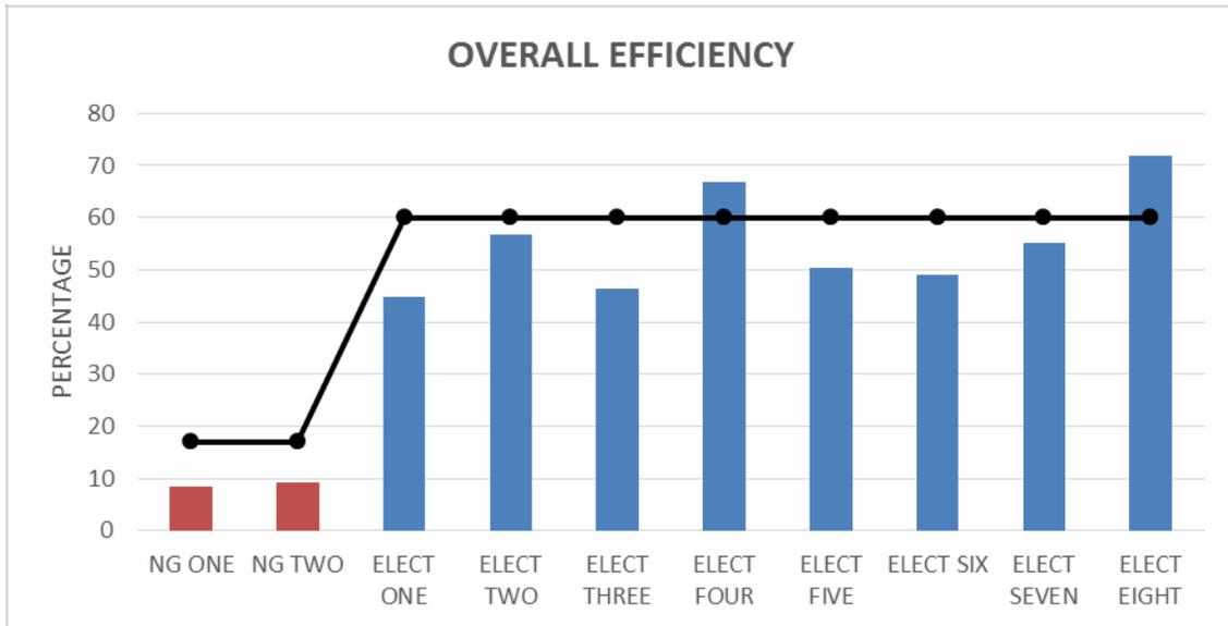
**Figure 4. Overall efficiency of the plant and pump compared to NPPPC acceptable efficiency (black line)**
