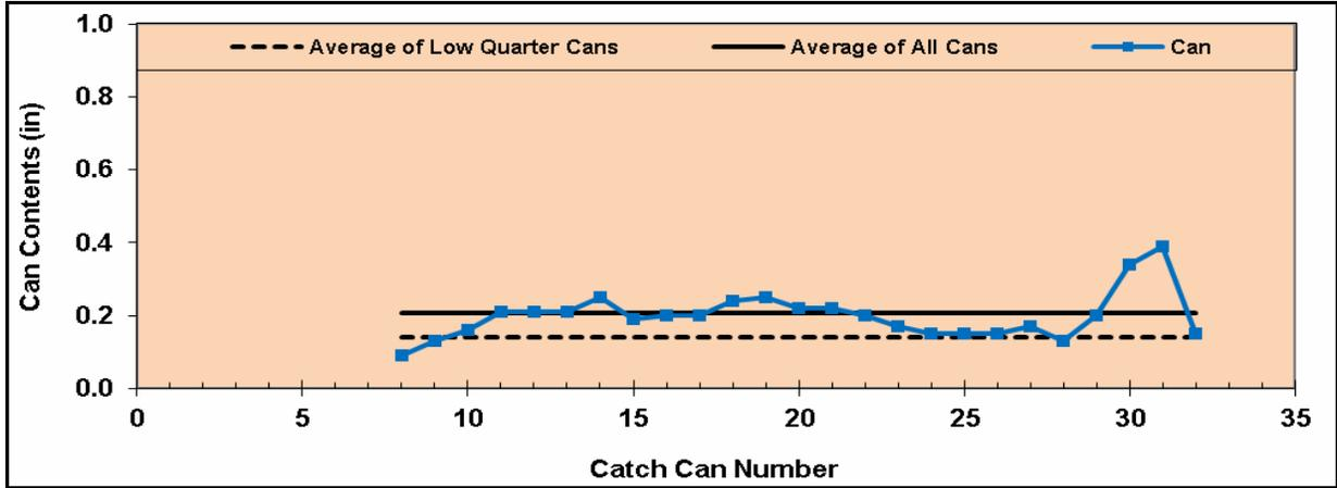
**Figure 2: Example of acceptable uniformity in tested Ogallala irrigation system**
