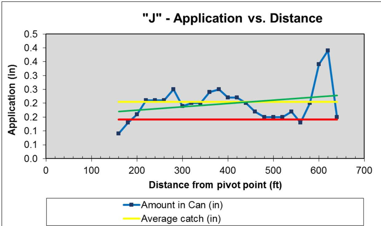
**Figure 7: Water application amount at distances from pivot**
