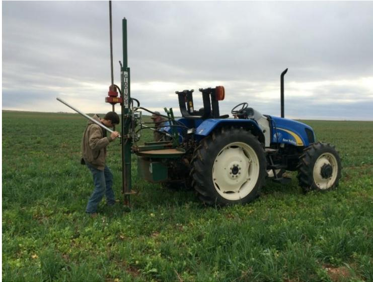
Figure 2. Soil coring device used in one of the study fields
