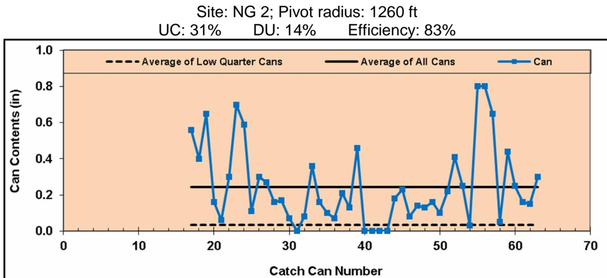
**Figure 1: Example of poor uniformity in tested Ogallala irrigation system**
