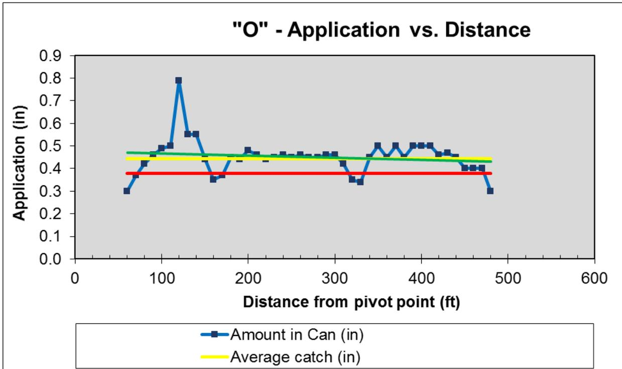
Figure 10: Water application amount at distances from pivot
